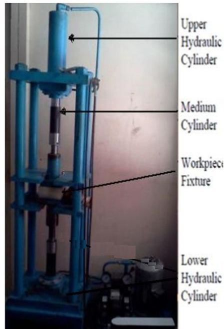
Figure- Two way abrasive flow machine
