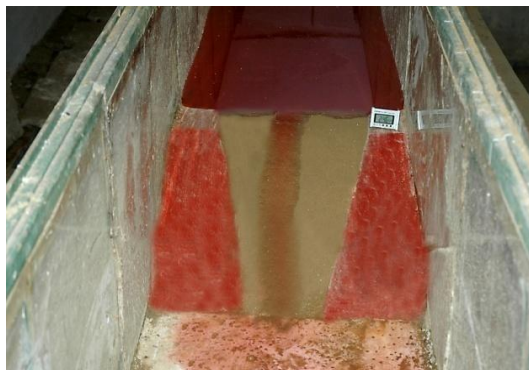
Figure 4b. Flow of water on fuse plug crest after overtopping.
