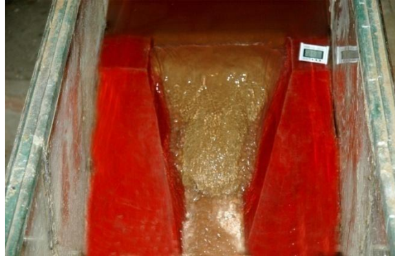
Figure 4d. Vertical of the breach of fuse plug and spillway type crest formation is seen.
