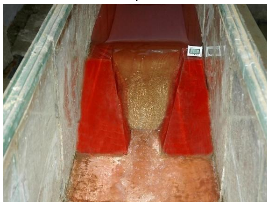
Figure 4c. Vertical cut in the downstream face of fuse plug along with receding of toe erosion in upward direction
