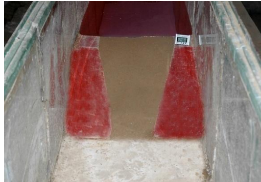
Figure 4a. Flow of water to the reservoir before overtopping the fuse plug model
