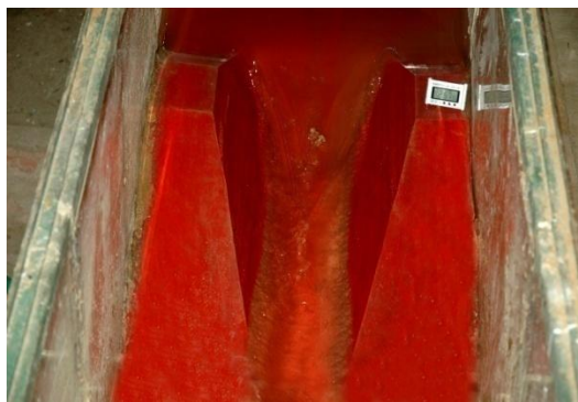
Figure 4e. Reduction in reservoir water level and total breaching process comes to final stage.
