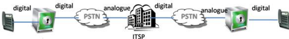
Figure9: ISDN VoIP (source: self-drawn, inspired by [4])
