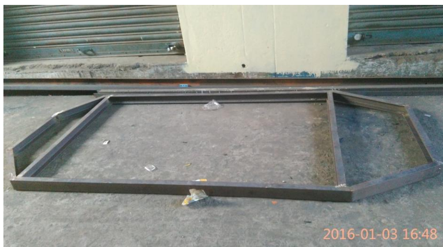
Fig .5.1: fabricated chassis with C cross section
