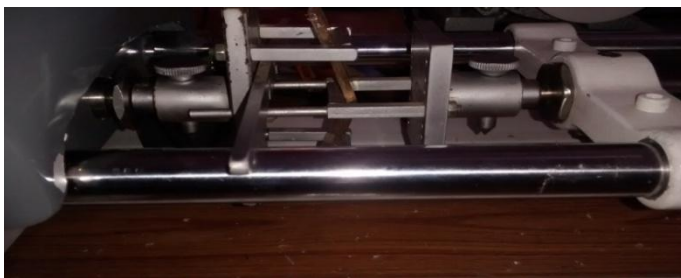
Figure 6 . 3 point bending test
