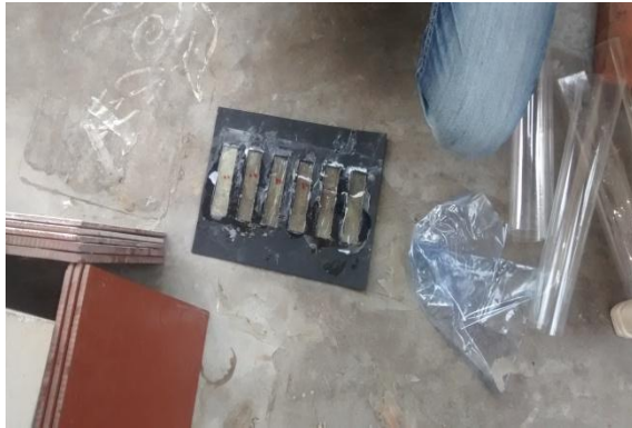
Figure 1 mould for preparing composites
