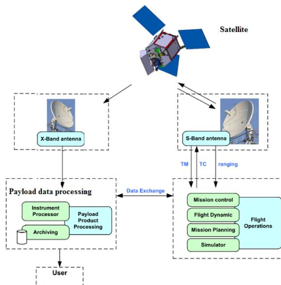
Fig. 1. Typical configuration of a remote sensing ground station
