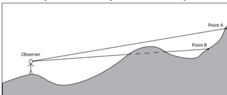
Fig 5. Visibility analysis. Point A is visible while Point B is not
