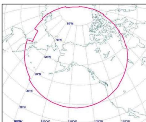
Fig 6. An example of a reception mask of ground station [2].
