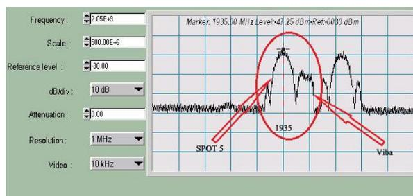
Fig.3. Unwanted signal detected in the MONRE's remote sensing station
