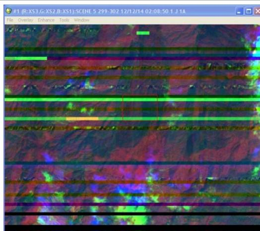
Fig.4. Noisy image caused by heavily impacted radio signal
