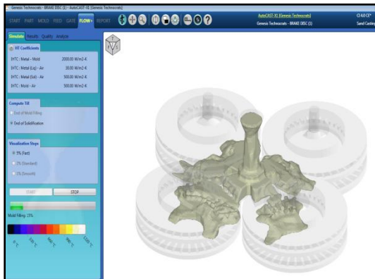
Fig.5. Mould filling at 20%
