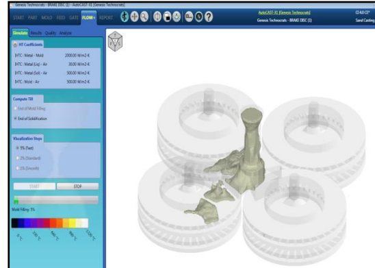
Fig.4. Mould filling at 10%
