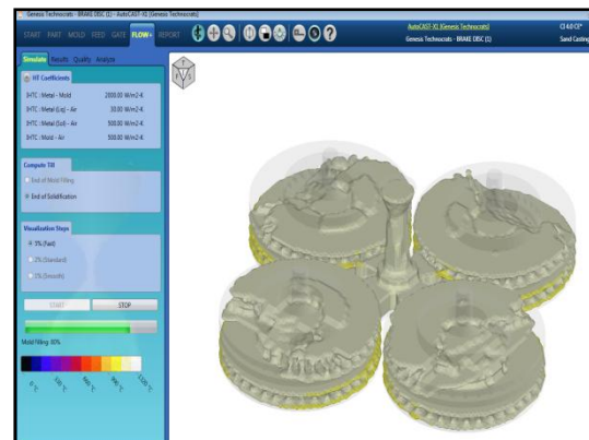
Fig.8. Mould filling at 80%
