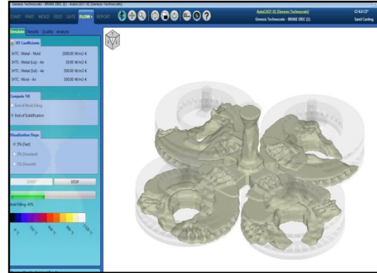
Fig.6. Mould filling at 40%
