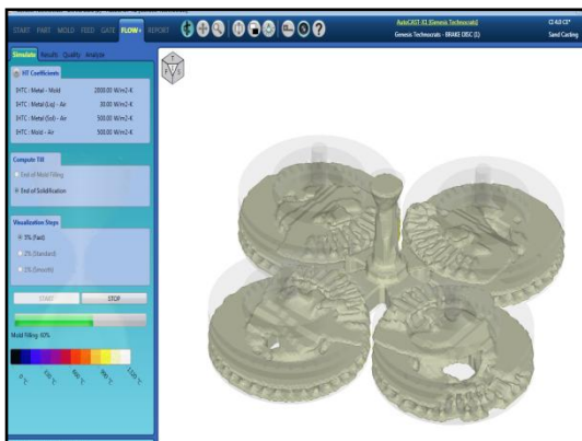
Fig.7. Mould filling at 60%
