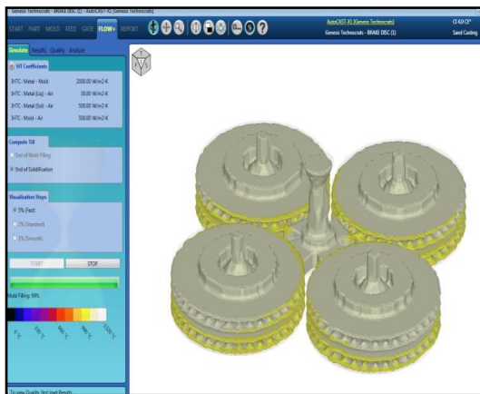
Fig.9. Mould filling at 100%
