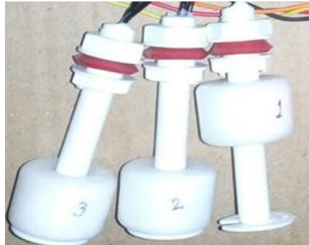
FIGURE 5: WATER LEVEL SENSORS
