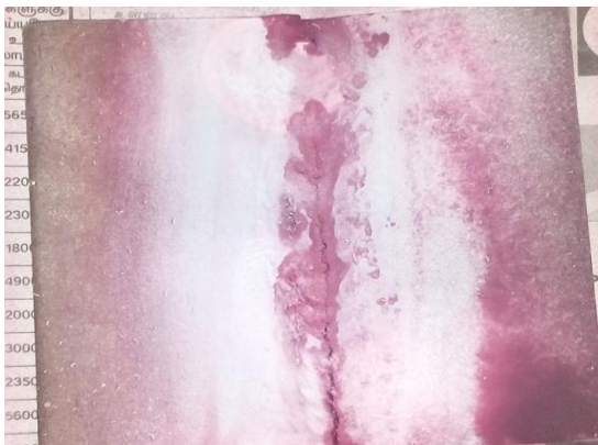
Penetrant test gas welding
