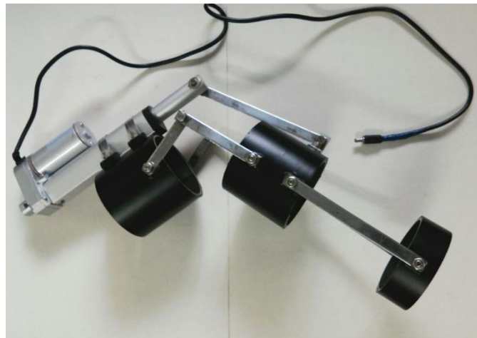
Figure 1: Exoskeleton framework with linear actuator.
