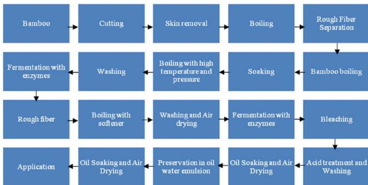
Figure 6 Extraction and treatment of rough and fine bamboo fibers (Source: Abdul Khalil(2012))
