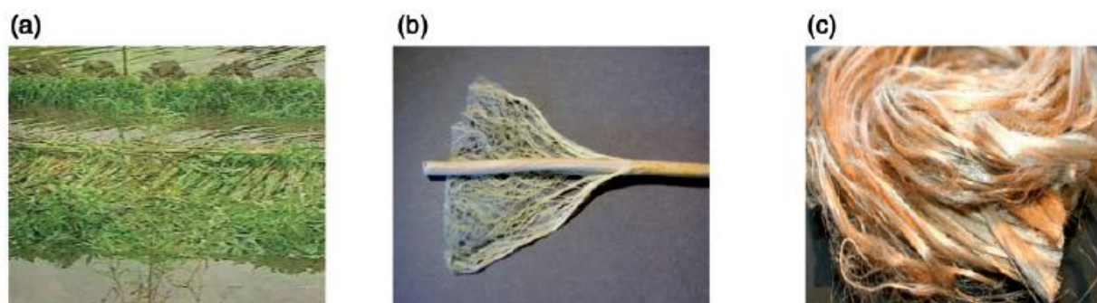
Figure 1 Kenaf fiber and its processing. (a) Kenaf water retting process, (b) kenaf stem showing fibers, (c) kenaf fiber (source: Kumar and Sekaran (2014))
