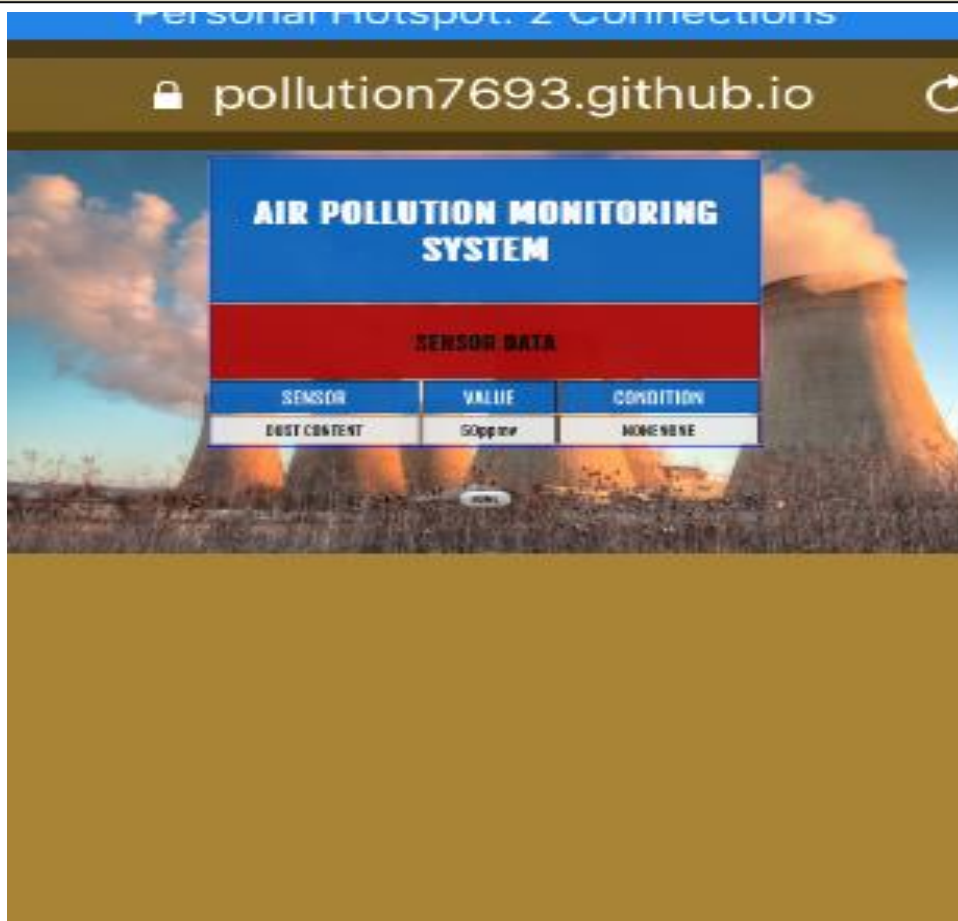
Screenshots of webserver displaying the status of each sensor.
