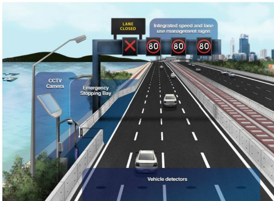
Fig. 7. Tulla freeway management system
