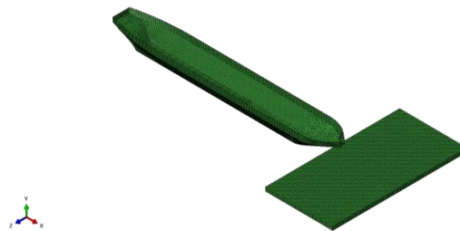
Fig.5 Finite element model of ship ice collision
